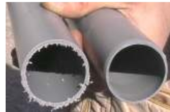
Plastic pipe, before and after cleaned with our rimmers.
